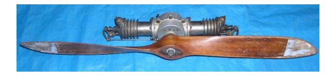
**YOU WANT OLD?** Here's old! It's a 1913 TW Clarke. It looks like a four stroke. And that prop says it's possibly used in pusher configuration. Although an early engine might be designed to turn either way, the prop in this case appears to be slightly concave on the near side, which could mean the prop turns "normally" or counter clockwise as we view it.
