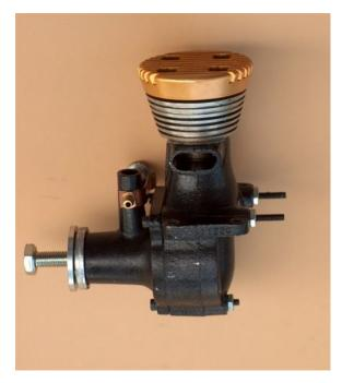
Here's the **Drone** diesel, one of the relatively few early US made diesels. Most Drones were sold in this configuration with a fixed compression head. But an accessory variable compression heads, as well as a glow heads were also available.
